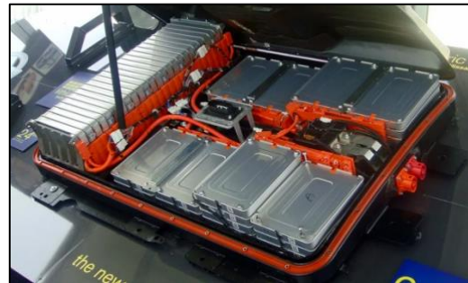
Nissan lithium battery pack
